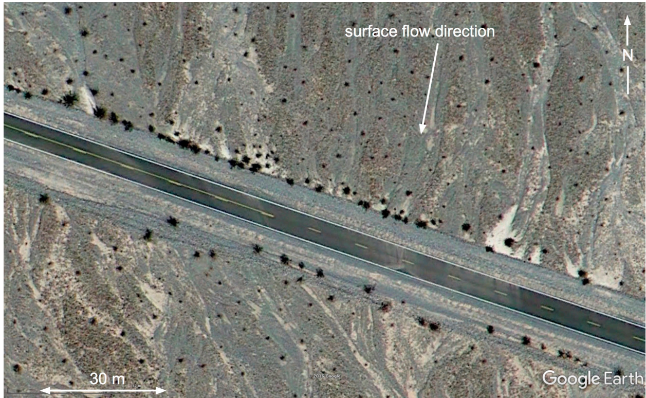
Figure 3. Google Earth image of a section of Scotty's Castle road. Enhanced creosote growth is obvious on either side of the road but it is more vigorous on the uphill ridge than on the downhill ridge. Also obvious immediately uphill of the uphill ridge are areas of light soil that are dried out ponded sediments, primarily clay. These occur because the uphill ridge acts as a barrier to surface flow on the fan. Note the absence of the dried up ponded sediments on the downhill side of the road. Stronger uphill growth and ponded sediments both occur most strongly when the flow direction is perpendicular to the road.
